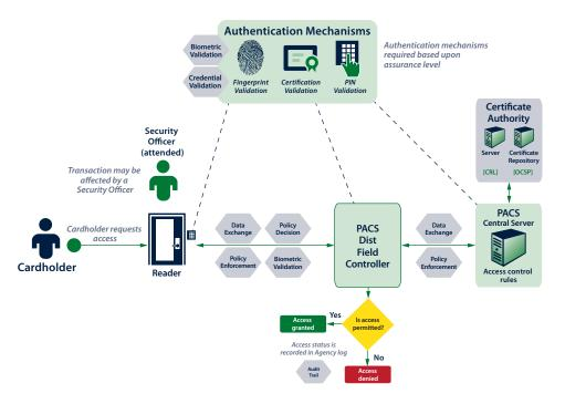
Figure 2 - Generic FPACS Functions based on Existing PACS Architectures
